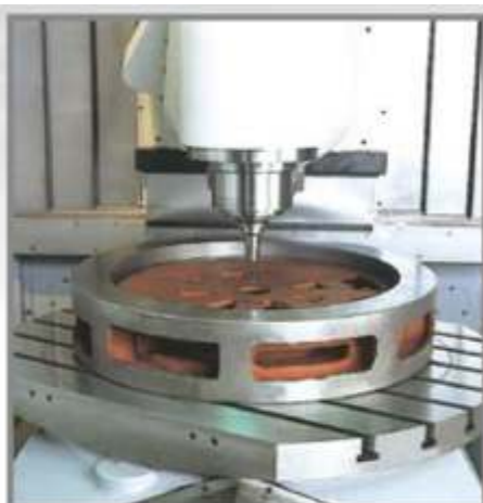
Automatic swiveling milling head
