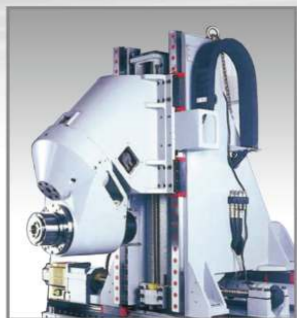
Automatic swiveling milling head
