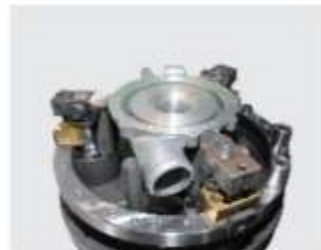
Motor part held in fixture
