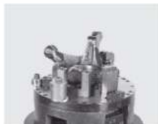
Stub axle held in fixture
