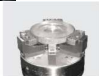
Fly wheel held in fixture
