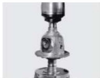
Diff case held in fixture with tailstock
