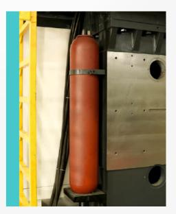
The Z-axis movement is effectively balanced through the use of dual hydraulic cylinders and a nitrogen accumulator. A bladder accumulator is strategically employed to equalize hydraulic pressure fluctuations, effectively mitigating the impact of sudden power failures.
