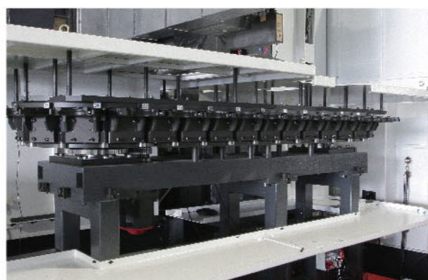
Tool magazine for 32, 48, 60 tool position
