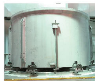
VTL3000ATC+C Wind power generator-stator machining
