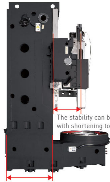
Thickness increased to guarantee structural rigidity.
