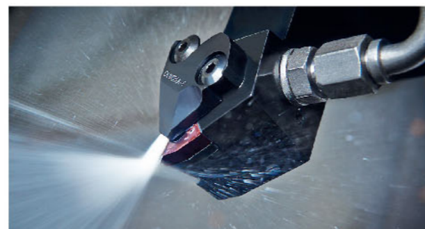
Coolant through tooling 12/20/60/ bar
